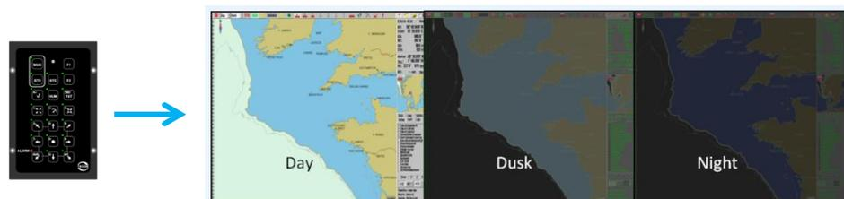
If you have a Furuno RCU-018 Keyboard or a TECDIS Keypad, we have now added support for cycling between day, dusk and night mode with the user-defined F1 and F2 keys. These keys are set in the auxiliary dropdown list in the Setup menu.
