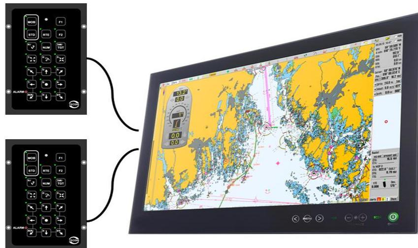
The biggest feature improvement in this release is the addition of a second connected TECDIS Keypad. This allows vessels with limited space to operate their primary TECDIS from two locations.
