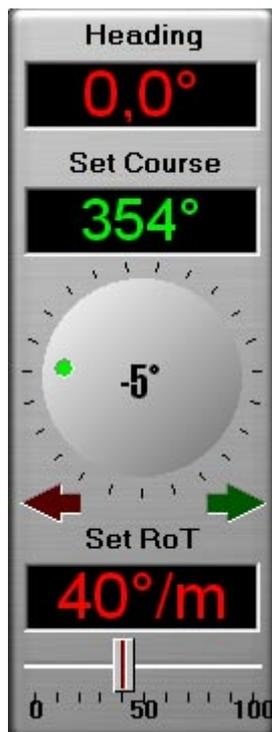
When the autopilot is set to External (remote) mode, a dialog is displayed in TECDIS, showing the current heading, the current Set Course and the current Set RoT (Rate of Turn).
