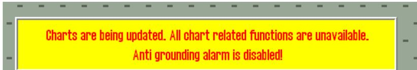
If the vessel is on screen when the update is applied, chart display is retained as long as the vessel remains on the screen, but it will not be possible to change scales or chart center position (or interact with the chart in any way) until either the vessel has moved off screen or the update is completed.
