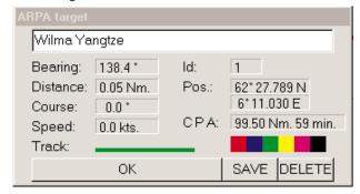
Placing the cursor on an ARPA-target and pressing the left button, an information window for the selected ARPA target will appear. Target name can be registered in this window. ARPAtracks can also be stored with date and selected colour.
