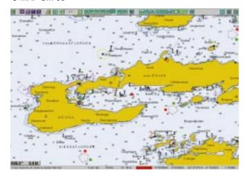
The TELchart ECS system makes use of the CM-93 chart presentation software developed along with the CM-93 database itself. It is important to notice that this increase the reliability and functionality in the computer system considerably by means of fast accessing of cartography and minimised demand of computer resources when displaying chart.
