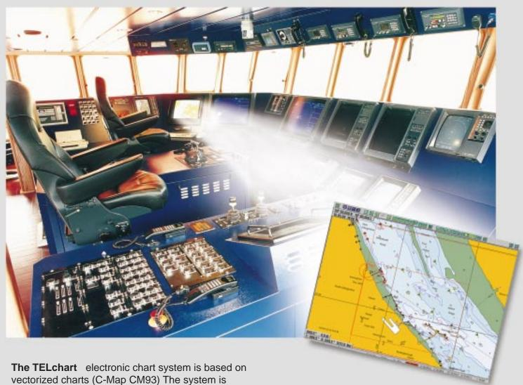
The TELchart electronic chart system is based on vectorized charts (C-Map CM93) The system is developed with an eye to simple operation and logical structure. At the same time it covers a wide variety of functions to satisfy requirements from demanding navigators.
