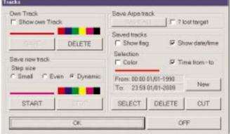
Own vessels track is always maintained. Track lines can be shown or hidden, and can be saved with selectable colour, text time and date. In addition tracks can easily be converted to routes.
