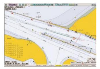
Vectorized cartography makes it possible to move from one chart to another without having to change chart display or storage media. All data is corrected to a common chart datum, WGS 84 as required by IMO and nescessary when using GPS as a position reference system.
