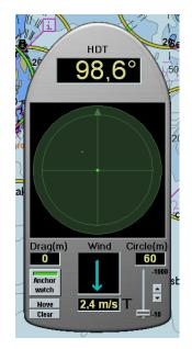
Note that the anchor watch feature now gives a warning when the ship is outside the turning radius of the anchor watch zone. This warning will be escalated to an alarm within 2 minutes if not acknowledged.
