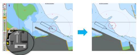
**To move the anchor position**: left click with the cursor on the center of the guard circle to select it, move the cursor to where you want the new center position to be, and then you place it there by left-clicking again.
